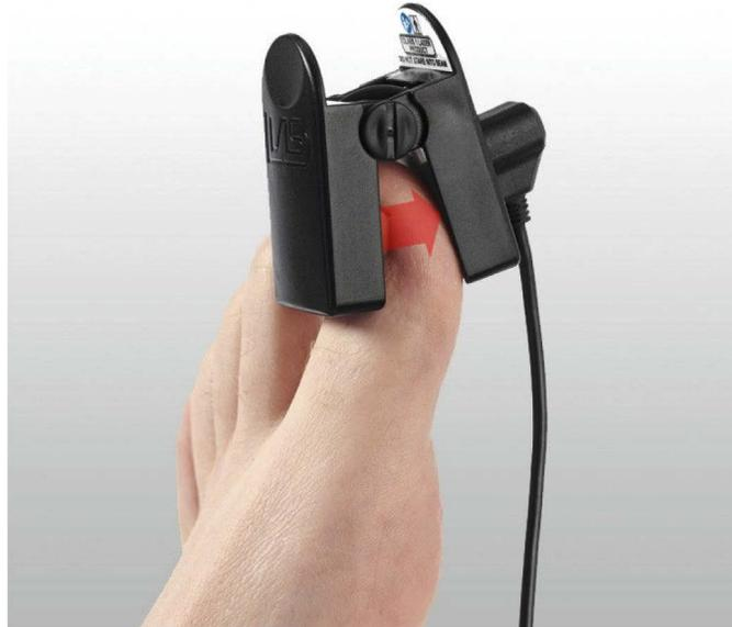
**Fig. 1.** Illustration of the SPG instrument clipped onto a subject's great toe. Coherent light from the laser diode scatters within the tissue (indicated by the red arrow) and is recorded by an image sensor on the opposing side.
